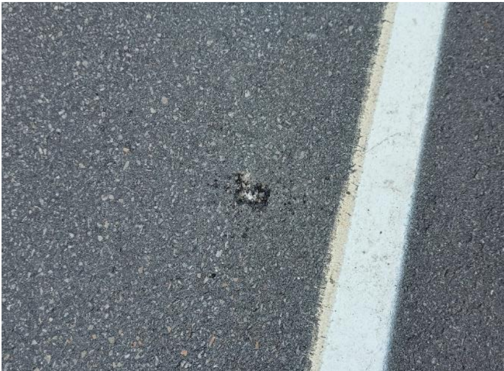
Photograph 46: Bridge No. 16-130-Highway 16 U/P. View of bulk asphalt sample 16-130-ASP-01A along top side of the bridge. All bulk samples collected from the Site found not to contain asbestos.
