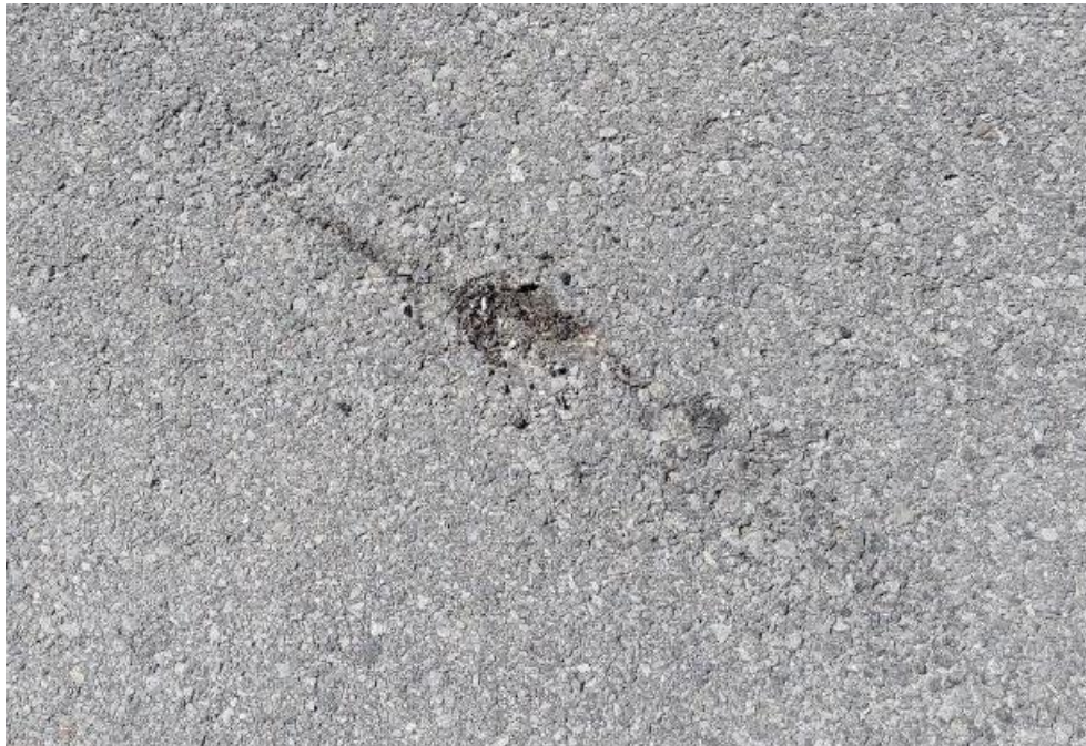
Photograph 10: Bridge No. 16-165 – Highway 401 Blue Church Road Underpass. View of bulk asphalt sample 16-165-ASP-01A along top side of the bridge. All bulk samples collected from the Site found not to contain asbestos.
