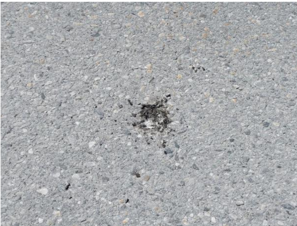
Photograph 42: Bridge No. 16-306 – Highway 401/416 W-N Ramp. View of bulk asphalt sample 16-306-ASP-01A along top side of the bridge. All bulk samples collected from the Site found not to contain asbestos.
